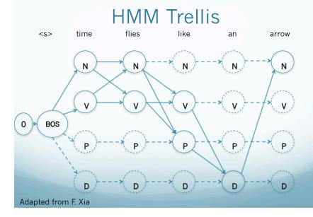
With a trellis you can keep track of all the sequence of tags possible, given a sentence, and write down the probabilities corresponding to the transitions and the emissions.
